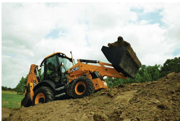
Figure 15-1: Cut and fill operations with the help of JCB
